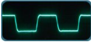
Figure 3 Square wave response at 10 kHz Measured by Tektronix CFG 253 Oscillator and KENWOOD CS-4125 Oscilloscope
